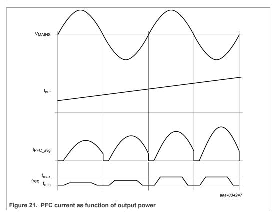
At the start of a mains cycle, the desired PFC current is zero and the PFC does not switch. When the PFC starts switching, the desired current is initially low and the PFC switching frequency is at minimum level. When the desired PFC current increases, the switching frequency increases as well until it reaches its maximum level.
