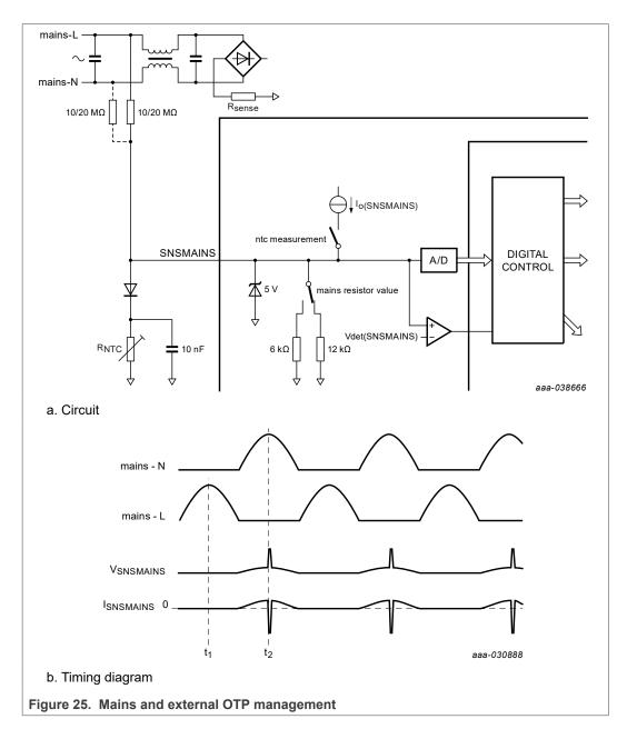
The TEA2017AAT continuously measures the SNSMAINS voltage via an A/D converter and waits until it detects a peak (t1). This peak value is internally stored and used for the mains compensation. The output of the A/D converter is used for brownout/brownin detection.
