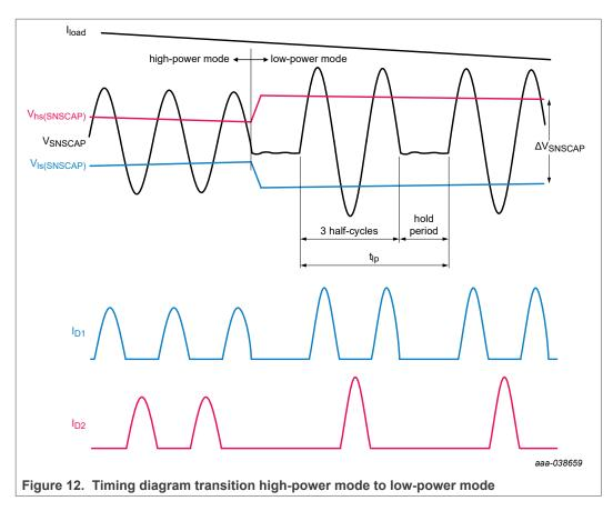
As the system continuously tracks the primary capacitor voltage, it knows exactly when to enter the "hold" period. It can also continue again at exactly the correct voltage and current levels of the resonant converter. In this way, a "hold" period can be introduced which reduces the magnetization and switching losses without any additional losses. The currents  $I_{D1}$  and  $I_{D2}$  (see Figure 12) are the secondary currents through diodes D1 and D2 (see Figure 7).
