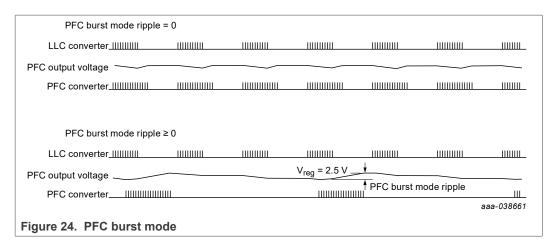
When the PFC is in burst mode and its output voltage drops to below the regulation level minus an adjustable ripple voltage, the PFC starts switching. When it reaches the regulation level again, the PFC stops switching.
