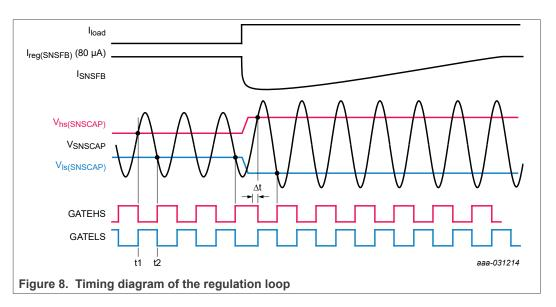
When the divided resonant capacitor voltage ( $V_{SNSCAP}$ ) exceeds the capacitor voltage high level ( $V_{hs(SNSCAP)}$ ), the high-side MOSFET is switched off (see <u>Figure 8</u> (t1)). After a short delay, the low-side MOSFET is switched on. Because of the resonant current, the resonant capacitor voltage initially increases further but eventually drops.
