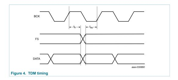
$L_{BST}$  = boost converter inductance;  $R_L$  = load resistance;  $L_L$  = load inductance. The TDM bit clock input (BCK) is used as a clock input for the amplifier and the DC-to-DC converter. The BCK and FS signals must be present for the [2] clock to operate correctly.
