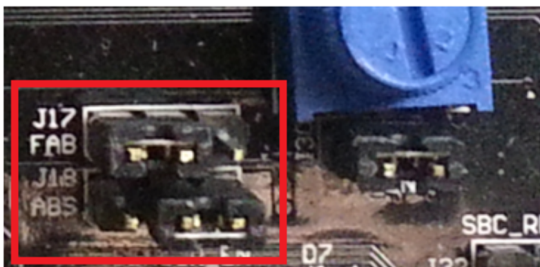
Figure 51. Jumper setting for Flash
