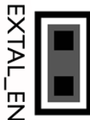
Figure 6-22: External Crystal Circuitry Enable (CT5)
