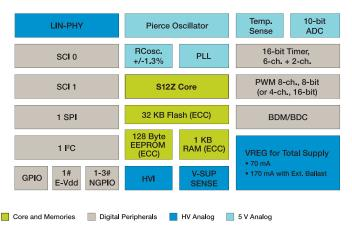
The MC9S12ZVL-Family is targeted at generic automotive applications requiring LIN connectivity. Typical examples of these applications include switches, actuators (e.g., window lift and door lock modules); body control electronics for occupant comfort (e.g., door, steering wheel, seat and mirror modules); and motors and sensors (e.g., in climate control, lighting, rain sensors, smart wipers, intelligent alternators and switch panels).
