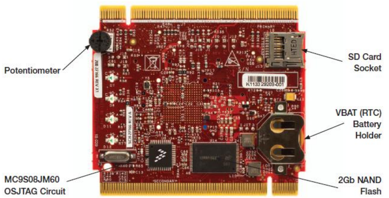
Figure 3. Callouts on back side of the TWR-K70F120M
