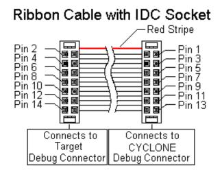
Figure 3-24: Ribbon Cable Example Diagram, When Looking Into IDC Socket
