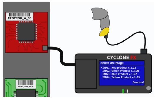
Figure 12-2: Bar Code Scanner On Production Line
