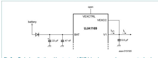
ig 5. Typical application without external PNP (showing example component values)
