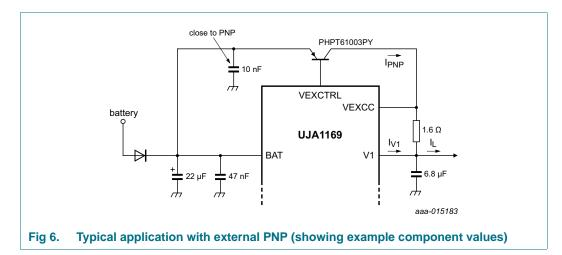
For short-circuit protection, a resistor must be connected between pins V1 and VEXCC to allow the current to be monitored. This resistor limits the current delivered by the external transistor. If the voltage difference between pins VEXCC and V1 reaches  $V_{th(act)llim}$ , the PNP current limiting activation threshold voltage, the transistor current will not increase further. In general, any PNP transistor with a current amplification factor ( $\beta$ ) of between 50 and 500 can be used.
