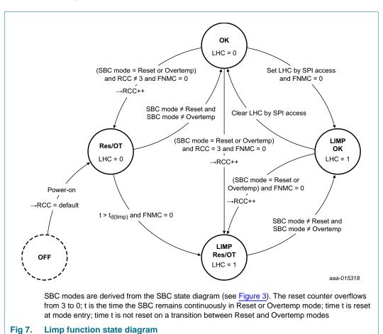
Note that the SBC always switches to Reset mode after leaving Sleep mode, since the SBC powers up V1 in response to a wake-up event. So RCC is incremented after each Sleep mode cycle. The application software needs to monitor RCC and update the value as necessary to ensure that multiple Sleep mode cycles do not cause the reset counter to overflow.
