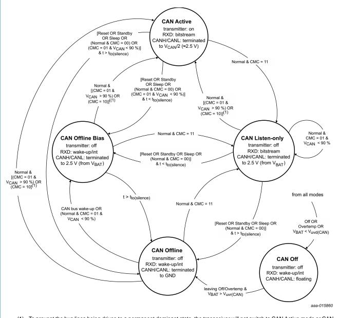
(1) To prevent the bus lines being driven to a permanent dominant state, the transceiver will not switch to CAN Active mode or CAN Listen-only mode if pin TXD is held LOW (e.g. by a short-circuit to GND)
