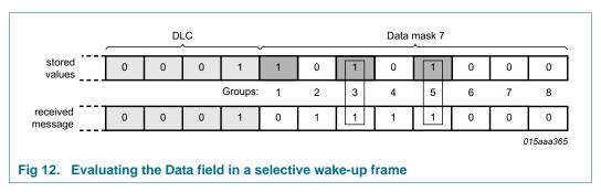
Optionally, the data length code and the data field can be excluded from the evaluation of the wake-up frame. If bit PNDM = 0, only the identifier field is evaluated to determine if the frame contains a valid wake-up message. If PNDM = 1 (the default value), the data field is included for wake-up filtering.
