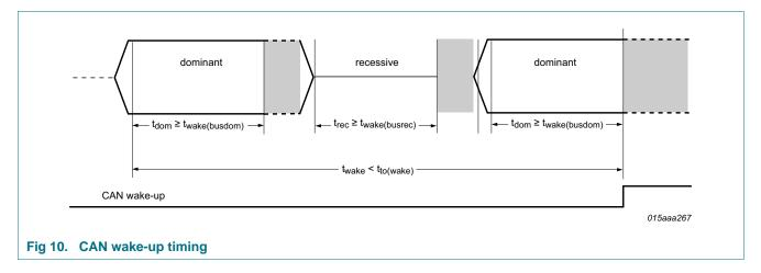
When a valid CAN wake-up pattern is detected on the bus, wake-up bit CW in the Transceiver event status register is set (see <u>Table 28</u>) and pin RXD is driven LOW. If the SBC was in Sleep mode when the wake-up pattern was detected, V1 is enabled to supply the microcontroller and the SBC switches to Standby mode via Reset mode.
