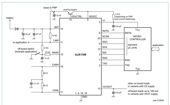
The application diagram contains example components and component values. A PHPT60603PY transistor could be used in place of the PHPT61003PY.
