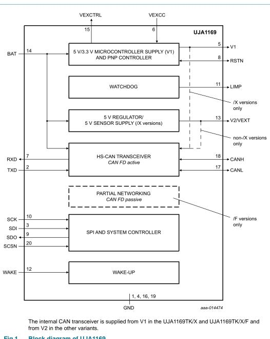
Fig 1. **Block diagram of UJA1169**
