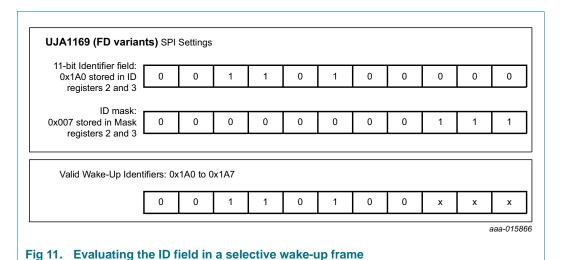
The data field indicates the nodes to be woken up. Within the data field, groups of nodes can be predefined and associated with bits in a data mask. By comparing the incoming data field with the data mask, multiple groups of nodes can be woken up simultaneously with a single wake-up message.
