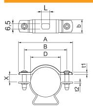
65,00 mm Dimension A Dimension B 51,00 mm 16,00 mm Dimension b 30,00 - 36,00 mm Dimension D Dimension D 36,00 mm 10,00 mm Dimension L 1,50 mm Dimension t1 1,50 mm Dimension t2 Dimension x 9,00 mm Distance to the wall  $\checkmark$ 1,00 Number of cables/pipes Version Closed Fastening type Screw hole Suitable in fire protection area  $\checkmark$  $\checkmark$ Halogen-free Plastic coated Clamping range D 30,00 - 36,00 mm
