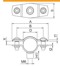
44,00 mm Dimension A Dimension B 32,00 mm 18,00 mm Dimension b 14,00 - 17,00 mm Dimension D Dimension D 17,00 mm Dimension H1 6,50 mm Dimension t1 1,00 mm 1,25 mm Dimension t2 Dimension x 4,50 mm Distance to the wall  $\checkmark$ 1,00 Number of cables/pipes Version Closed Fastening type Threaded connection  $\checkmark$
