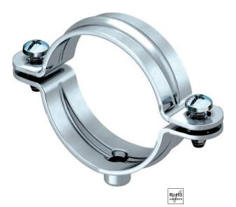
Mounting with screw-in spacer clips. Spacer clips and screw-in spacer clips are available in various materials: in V2A stainless steel, in electrogalvanised, hot-dip galvanised steel or in aluminium. Fastening can take place with bolt ties or angler anchors and Sprint screws. Depending on the design, the clips can be "shot" using a bolt-firing tool or nail device.
