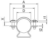
59,00 mm Dimension A Dimension B 45,00 mm 16,00 mm Dimension b 25,00 - 30,00 mm Dimension D Dimension D 30,00 mm Dimension L 10,00 mm Dimension t1 1,50 mm 1,50 mm Dimension t2 Dimension x 7,50 mm Distance to the wall  $\checkmark$ 1,00 Number of cables/pipes Version Closed Fastening type Screw hole Suitable in fire protection area  $\checkmark$  $\checkmark$ Halogen-free Plastic coated Clamping range D 25,00 - 30,00 mm
