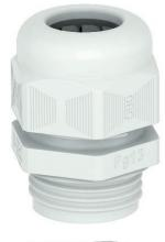
The quickest and most convenient way of providing strain relief and tightness with cable glands on junction boxes and housings is with the tried-and-trusted V-TEC VM cable glands from OBO. With the integrated sealing lip and the special OBO slat technology, protection class IP68 is achieved. Strain relief and tightness have been tested to DIN EN 62444.
