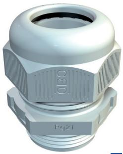
The quickest and most convenient way of providing strain relief and tightness with cable glands on junction boxes and housings is with the tried-and-trusted V-TEC VM cable glands from OBO. With the integrated sealing lip and the special OBO slat technology, protection class IP68 is achieved. Strain relief and tightness have been tested to DIN EN 62444.
