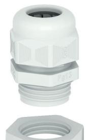
The quickest and most convenient way of providing strain relief and tightness with cable glands on junction boxes and housings is with the tried-and-trusted V-TEC VM cable glands from OBO. With the integrated sealing lip and the special OBO slat technology, protection class IP68 is achieved. Strain relief and tightness have been tested to DIN EN 62444.
