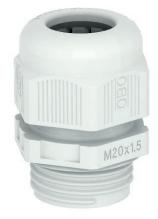
The quickest and most convenient way of providing strain relief and tightness with cable glands on junction boxes and housings is with the tried-and-trusted V-TEC VM cable glands from OBO. With the integrated sealing lip and the special OBO slat technology, protection class IP68 is achieved. Strain relief and tightness have been tested to DIN EN 62444.
