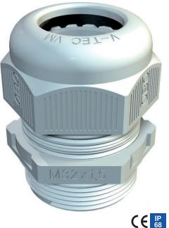
The quickest and most convenient way of providing strain relief and tightness with cable glands on junction boxes and housings is with the tried-and-trusted V-TEC VM cable glands from OBO. With the integrated sealing lip and the special OBO slat technology, protection class IP68 is achieved. Strain relief and tightness have been tested to DIN EN 62444.
