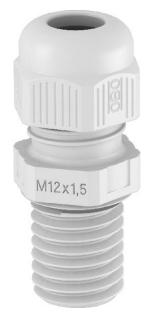
The quickest and most convenient way of providing strain relief and tightness with cable glands on junction boxes and housings is with the tried-and-trusted V-TEC VM cable glands from OBO. With the integrated sealing lip and the special OBO slat technology, protection class IP68 is achieved. Strain relief and tightness have been tested to DIN EN 62444.
