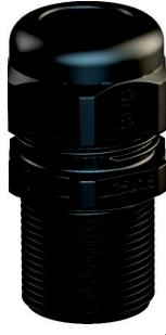
The quickest and most convenient way of providing strain relief and tightness with cable glands on junction boxes and housings is with the tried-and-trusted V-TEC VM cable glands from OBO. With the integrated sealing lip and the special OBO slat technology, protection class IP68 is achieved. Strain relief and tightness have been tested to DIN EN 62444.
