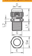
Dimension E 60,00 mm Dimension L min. 37,50 mm 54,30 mm Dimension L max. 24,00 mm Dimension L1 Dimension L2 8,00 mm SW 54,00 mm Version Straight Type of seal Sealing ring Bend protection  $|\times|$ Sealing range D 23,00 - 35,00 mm
