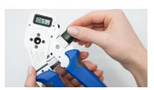
Positioner for 080.000.072.000.000: Insert the positioner into the crimping tool. To do this, turn the tool around so that the rear side is facing you. Insert the positioner with bayonet pin into the adapter ring and turn 90°. The positioner locks into place.
