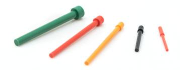
Sealing plugs are used to seal unwired contact cavities. After installing unwired contacts into unused cavities, insert knob end of sealing plug into grommet until it bottoms against the unwired contact per illustration. Install sealing plugs with standard contact insertion / extraction tools.
