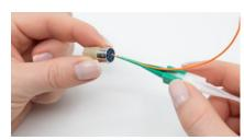
Insert the contacts until you feel them click into place in the retaining clip. If required, check that the contact is firmly seated by gently pulling on it. Remove the tool by sliding it back on the wire.
