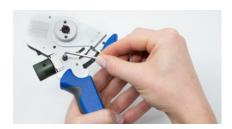
Set the crimp dimension to the desired level with the crimp setting adjustment wheel and then fix the clamping screw.
