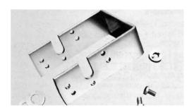
Ohmite coupling kits permit tandem mounting of two rheostat units. A coupling fastens to the shaft of the back unit; projections on the coupling engage the recesses in the driving hub of the front unit.
