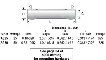
Ohmite now offers the Audio Gold Resistor Family, specifically designed for high-end loudspeaker and amplifier applications. These resistors utilize high quality resistance wire wound on a ceramic core, terminated, and finished with our flameproof Centohm® coating.
