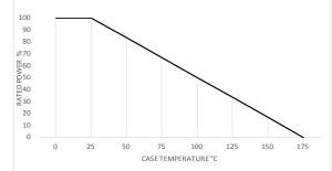
The case temperature is to be used for the definition of the applied power limit The case temperature measurement must be made with a thermocouple contacting the centre of the component mounted on the designed heat sink Thermal grease should be applied properly
