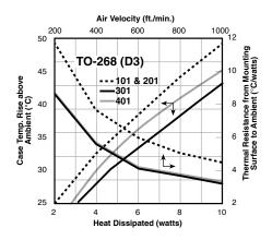
Final thermal performance is highly dependent on the thermal characteristics of the PCB. It is possible to see a 50% drop in temp rise in natural convection with a thermally improved PCB.
