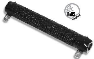
Corrib<sup>®</sup> resistors are ideal for applications involving high currents at very low resistance values—as low as  $0.1\Omega$  for the 300 Watt unit. These large, heavyduty resistors are designed to withstand frequent start-stop cycles characteristic of motor starting, dynamic braking and other similar applications. Special order units are available to accommodate up to 1500 watts.
