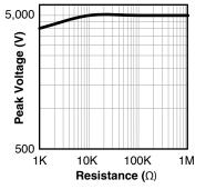
Resistors are tested in accordance with IEC61000-4-5, waveform 1.2/50 $\mu$ S, 10 Pulses applied. Limit of acceptance is a shift in resistance of less then 1% from the initial value. Graph data shows values equal or greather than 1K $\Omega$ .
