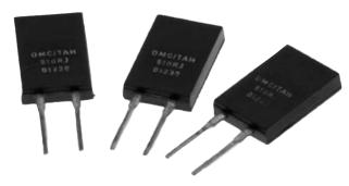
The TAH20 is a completely encapsulated thick film resistor in the TO220 package outline. Rated for 20 watts @ 25°C case temperature, these resistors are electrically isolated, and molded in a high temperature case.
