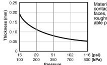
Material compressibility improves contact between the mating surfaces, adjusting for flatness and roughness variations, ensuring reliable performance.
