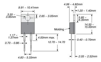
Note: These dimensions apply to TBH products manufactured after June 10, 2016
