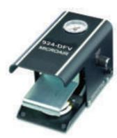
The 924-DFV Series Foot Valve Dispenser offers increased production combined with dispenser economy. Floor mounted, they have a built in pressure regulator, pressure gauge and a unique fast-dump, three-way air valve. Output rate and shot size are operator controlled.
