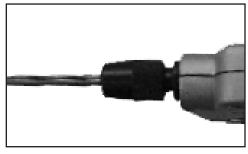
Place sleeve over the bit and slide the sleeve into the nose piece. Rotate the sleeve as you are sliding the sleeve into the nose piece until the sleeve has engaged with the collet pin, the sleeve will then slide further into the nose piece. The sleeve is now seated.
