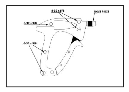
Turn the gun over and lay it down on a flat surface so the nose piece is facing left. Separate the housings and remove the collet and nose piece. Note: Use a flat head screwdriver to separate the housings. 3. Apply grease to the bevel, spur and face gear.
