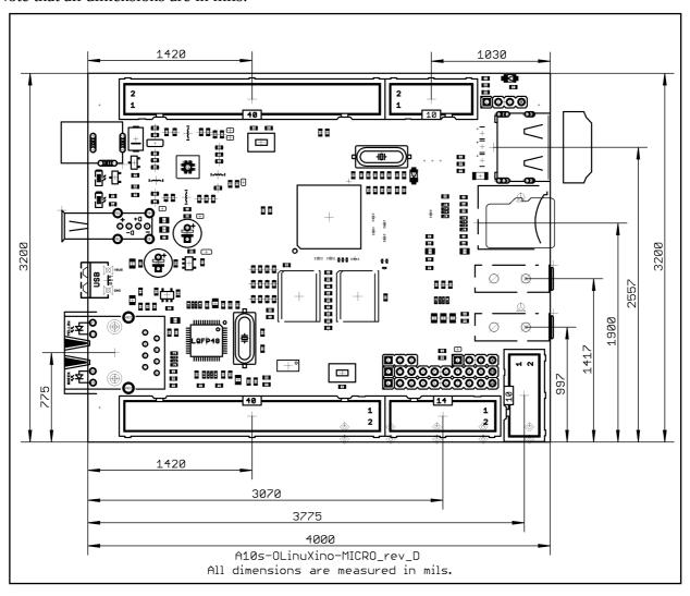
The three highest elements on the board in order from the tallest to the shortest are: USB\_HOST connector -650mils, the Ethernet connector -600mils, capacitors C86/C94 - 525mils
