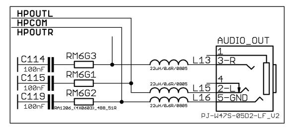
The connector can interface standard 3.5 mm phone connector (also known stereo plug or audio plug).
