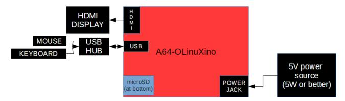
**1.2.5** Power the display and apply the power supply to the board. The graphical user interface should start automatically. By default the super user name is "root" the password is "olimex".
