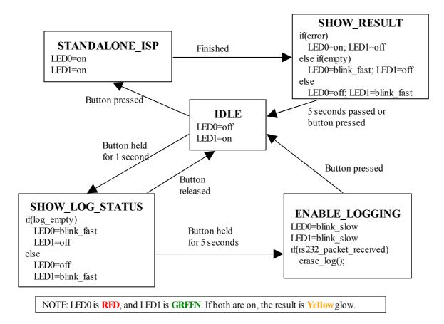
In case of autonomous operation error, the RED LED will blink for a while. The number of flashes indicates the error that caused the failure. Error codes are given in the table below.
