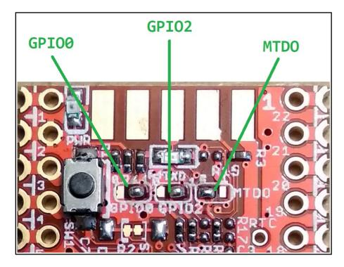
The jumpers for the default FLASH mode were set during production as follows: GPIO0 is set to position 1; GPIO2 is set to position 1; MTD0 is set to position 0.
