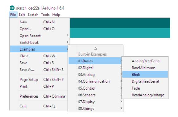
A new window with code would open. Edit the code in order to reflect the hardware of ESP8266-EVB boards. By default, the example assumes the LED is connected to digital pin #13 (like in most Arduino boards). In our case the relay that has a LED is connected to digital pin #5. This information can be acquired from the schematic of the board. Replace all occurrences of "13" with "5". The code should look as follows:
