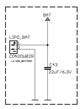
The iMX233 has a built-in battery recharge circuit. This means that if you have a battery and external power supply connected simultaneously, if the battery is not fully charged it would start charging (drawing current from the external power supply).
