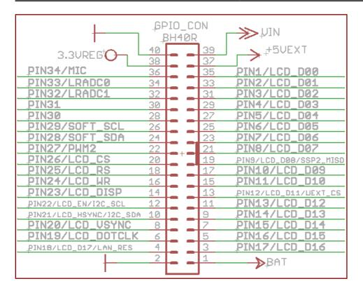
When looking at the bottom of OLinuXino-MAXI near the GPIO connector there is also an additional GND pad named GND\_PIN which is a fast way to have access to a ground signal.
