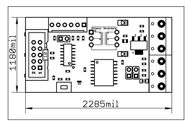
The three highest elements on the board in order from the tallest to the shortest are: ICSP connector – 450mils, RS485 connector – 400mils, UEXT connector – 350mils.
