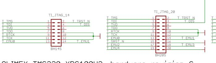
OLIMEX TMS320-XDS100V3, hardware revision C DEBUG HEADER LAYOUTS
