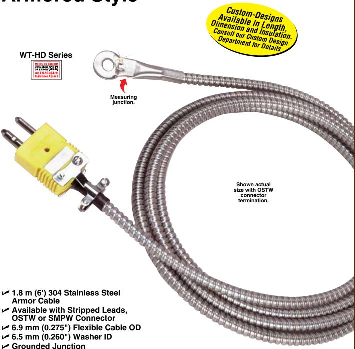
Rugged thermocouple, for surface mount applications, has a washer mounting surface and an overall dimension of 17.3 mm (0.680") OD, with a 6.6 mm (0.260") mounting hole of 304 SS material. Attached to the mounting surface: 1.8 m (6') of 304 SS flexible armor cable with stripped wire ends. Armor cable has 6.9 mm (0.275") OD, with 1.78 mm (0.070") washer thickness. Standard male connectors are available for cold-end termination. Rated to 480°C (900°F) for Type K only.
