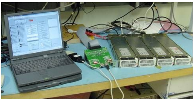
Figure 10 -Test setup using a OmniOn J85480 shelf
