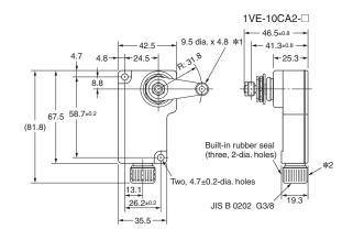
\*1. The stainless steel roller arm can be set to any position within 360°. \*2. Conduit cap.
