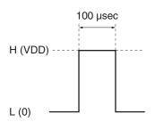
Examples of the reset pulse (reset at the potential of High)
