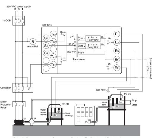
**Automatic Water Supply Control with Pump Idling Prevention**
