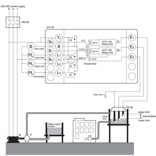
Note: 1. Be sure to ground the common Electrode E3 (the longest Electrode).
