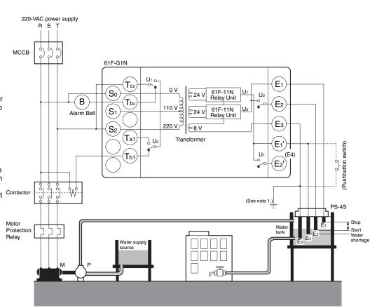
**Automatic Water Supply Control with Abnormal Water Shortage Alarm**
