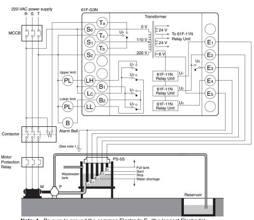
**Note: 1.** Be sure to ground the common Electrode  $E_5$  (the longest Electrode).
