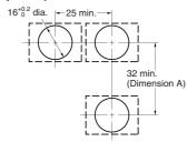
Note: 1. Make sure the thickness of the mounting panel is 0.5 to 3.2 mm. If, however, a Switch Guard or Dust Cover is used, the thickness of the mounting panel must be 0.5 to 2 mm.
