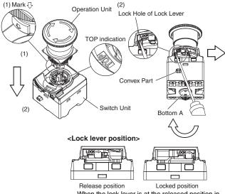
When the lock lever is at the released position in this Switch, the NO and NC contact operation is reversed.
