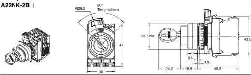
**Three-position Switches with Plastic Bezels**
