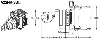
Two-position Switches with Brushed Metal Bezels Three-position Switches with Brushed Metal Bezels
