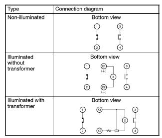
Note: The above terminal connection diagrams are examples for SPST-NO + SPST-NC.
